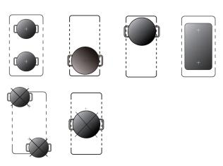
1. To activate the flexible area as a single big zone, simply press the **same time** related heating zone power slider regulating key at least 2 second
