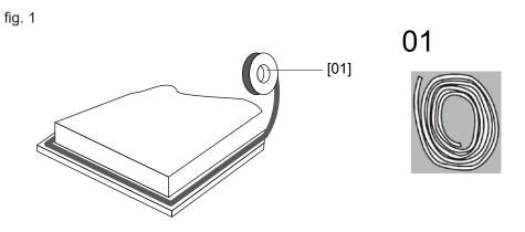
Stretch out the supplied seal along the underside edge of the hob, ensuring the ends overlap.
