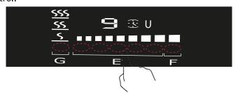
4. If the pot is moved from the front to the rear part (or viceversa), the flexible area detects automatically the new position, keeping the same power.
